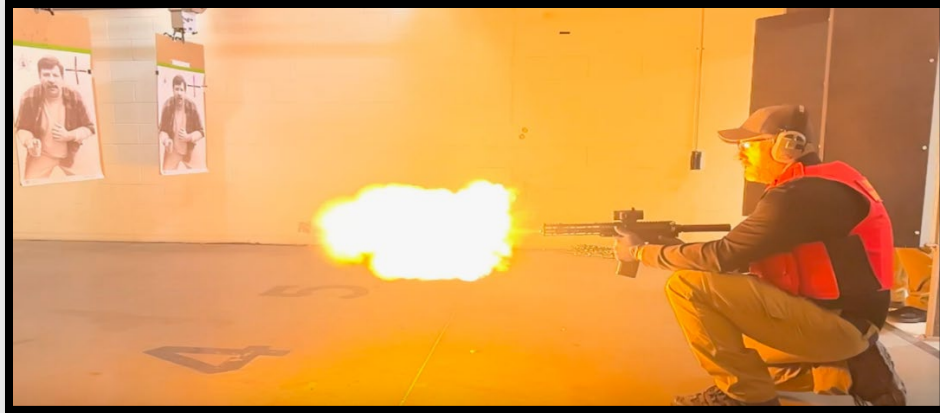
Test Firing of confiscated AR-15 Pistol from criminal case for NIBIN analysis
